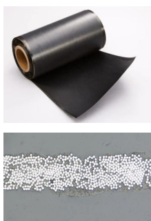
Cross-section image of UD tape
