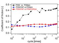
POM/CNF has excellent sliding properties even between the same material and under greaseless conditions.
